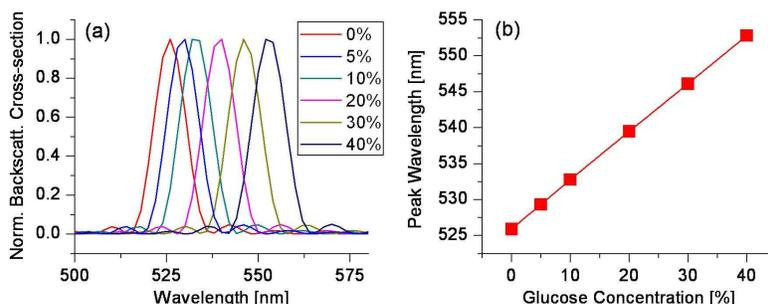
Fig. 5. Theoretical calculation for refractometric sensing with periodic silk gratings: (a) Normalized back-scattering cross-section of a grating composed of 256 100nm-radius silk spheres with a lattice constant of 600 nm immersed in water and glucose solutions and illuminated by a plane wave at 10 degrees to the array plane; (b) Shift of the peak wavelength as a function of the glucose concentration in the solution.
