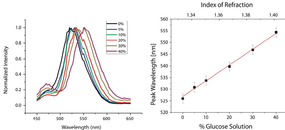
Fig. 4. Experimental structural color change with varying refractive index. (a) Spectra of the 400 nm lattice constant structure illuminated with supercontinuum with different concentrations of glucose. (b) Plot of the peak in (a) vs. glucose concentration and index of refraction.
