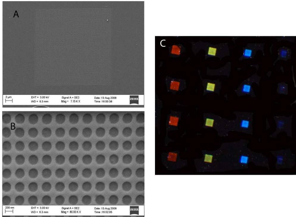
Fig. 1. A. SEM image of periodic nanoholes in silk. The nanoholes are 200 nm in diameter, 30 nm deep and separated by 300 nm. B) Magnified image of A. C) Periodic nanoholes in silk illuminated with light from a dark-field condenser. The lattice constants are from left to right 700, 600, 500, and 400 nm. The distance between the rows of colored squares is 200  $\mu\text{m}$ .
